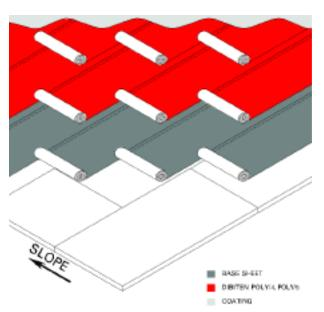
laps must be rolled with a 3" (76 mm) rounded edge roller. A 1/8" to 3/8" (3 mm to 10 mm) bleedout of compound shall be visible at the edge of all seams. All laps must be checked for good adhesions.
