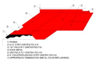
Note: STEP 8, not shown, is the installation of walking deck surfacing such as tiles, heavy duty outdoor carpeting, or similar appropriate materials suitable for protecting the Dibiten membrane from puncture. (A loose laid ply sheet (such as 11 lb. fiber glass) is required between the 2nd layer of Poly/4 and the decking material unless outdoor carpeting is used, in which case a water-based adhesive compatible with the Dibiten membrane must be used).
